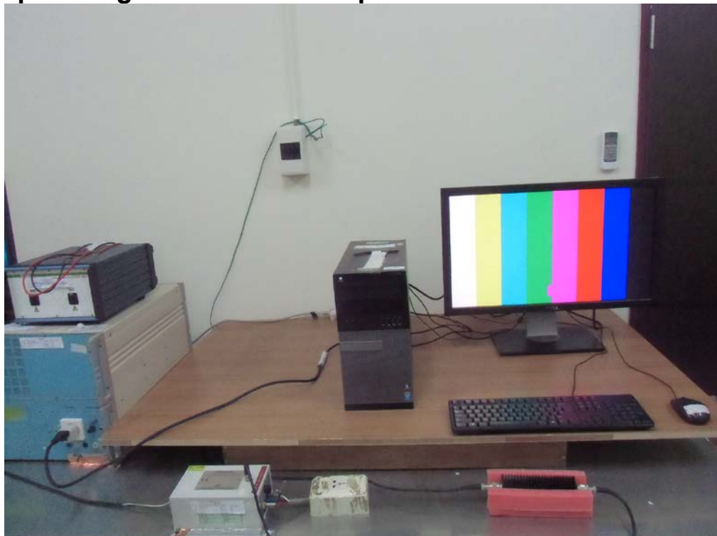
Photograph –Surge & EFT Test Setup
