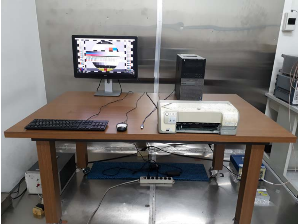
Photograph – Conducted Emission Test Setup
